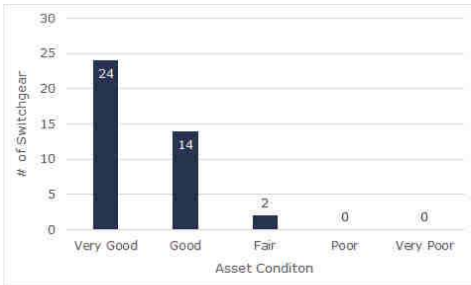
Figure 3-10: Condition Assessment Results for Pad-mounted Switchgear
