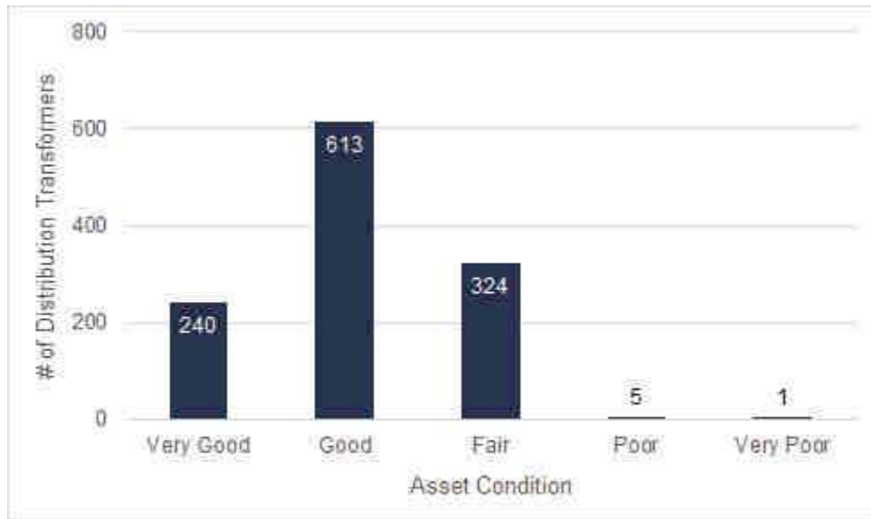
1 Figure 3-13: Condition assessment results for pole-mounted transformers
