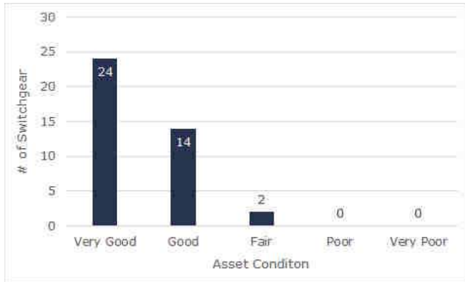
Figure 3-15: Condition assessment results for pad-mounted switchgear
